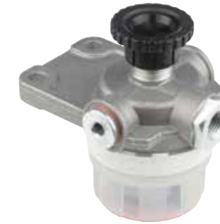
50-22071 MERCEDES OTOBÜS EL OTOMATİĞİ MB BUS HAND PUMP Mercedes Ref. 000 090 73 50
