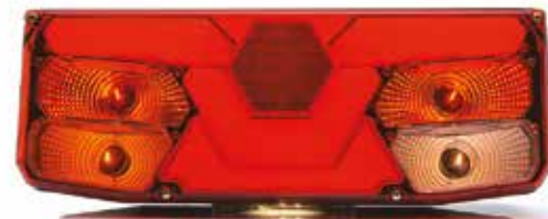
62-1053 HİBRİT / HYBRID SOL / LEFT 12-24V IP56 5 Fonksiyon: Pozisyon, Stop, Sinyal, Geri Vites, Sis 5 Functions: Position, Stop, Indicator, Reverse, Fog 62-1053KL CAM / LENS
