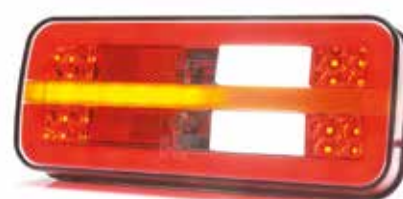
62-1324DDL LED SOL-SAĞ / LEFT-RIGHT 12-24V IP66/68 5 Fonksiyon: Pozisyon, Stop, Sinyal, Geri Vites, Sis 5 Functions: Position, Stop, Indicator, Reverse, Fog
