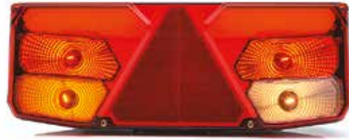
62-1029 HİBRİT / HYBRID SOL / LEFT 12-24V IP56 5 Fonksiyon: Pozisyon, Stop, Sinyal, Geri Vites, Sis 5 Functions: Position, Stop, Indicator, Reverse, Fog 62-1029KL CAM / LENS
