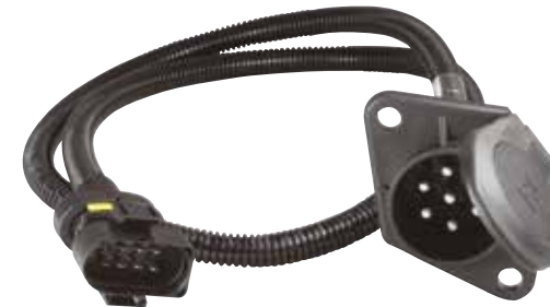
61-511119 7'Lİ ADAPTÖR KABLO, N TİPİ, 24V, 1,1m, ISO 1185'E UYGUN 7 PIN ADAPTER CABLE, N TYPE, 24V, 1,1m, ACC. ISO 1185 OE 81.25432.6201 81.25432.6182
